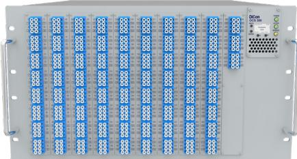
**DiCon OCS-300** is a high-density, 300x300 fully non-blocking **Optical Circuit Switch (OCS)** engineered specifically to meet the cost expectation and rigorous performance demands of AI data center networks. Built on DiCon's proprietary **MEMS mirror technology**, this matrix switch leverages a platform that has been in high-volume commercial deployment for more than 20 years, offering an unrivaled track record of field-proven reliability.
